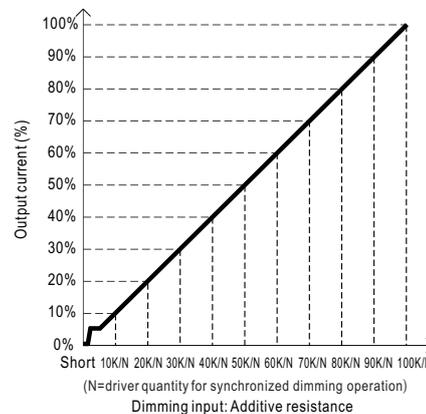
Note : 1. Min. dimming level is about 8% and the output current is not defined when 0% < I<sub>out</sub> < 8%.
